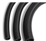
Hose: Evaflex polyurethane, antistatic, heat resistant up to 120° C oilproof Ø50 mm
