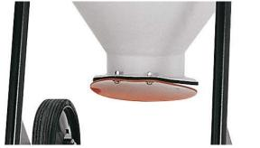
Creates a vortex of the incoming dust helping to keep the filter clean. In addition, it is equipped with a vacuum inlet seal to prevent
