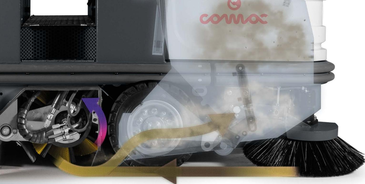
The pressure and height adjustment of the central brush are controlled simply by the knob near the brush. Brush height adjustment depending on wear can, therefore, be done very easily. This ensures a longer brush life cycle.
