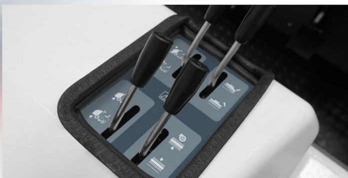
The controls and motors fitted on the CS100/CS120 models are hydraulically operated to guarantee reliability and ease of use.
