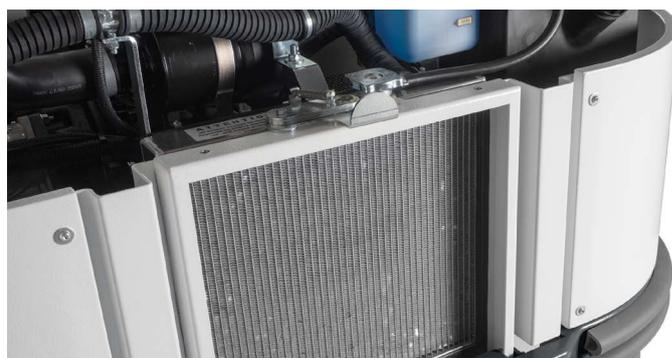
All models feature an oil cooler with independent thermostat and solenoid valve in order to keep oil temperature within the ideal range and ensure best efficiency. In this way consumption is reduced and components' life extended.
