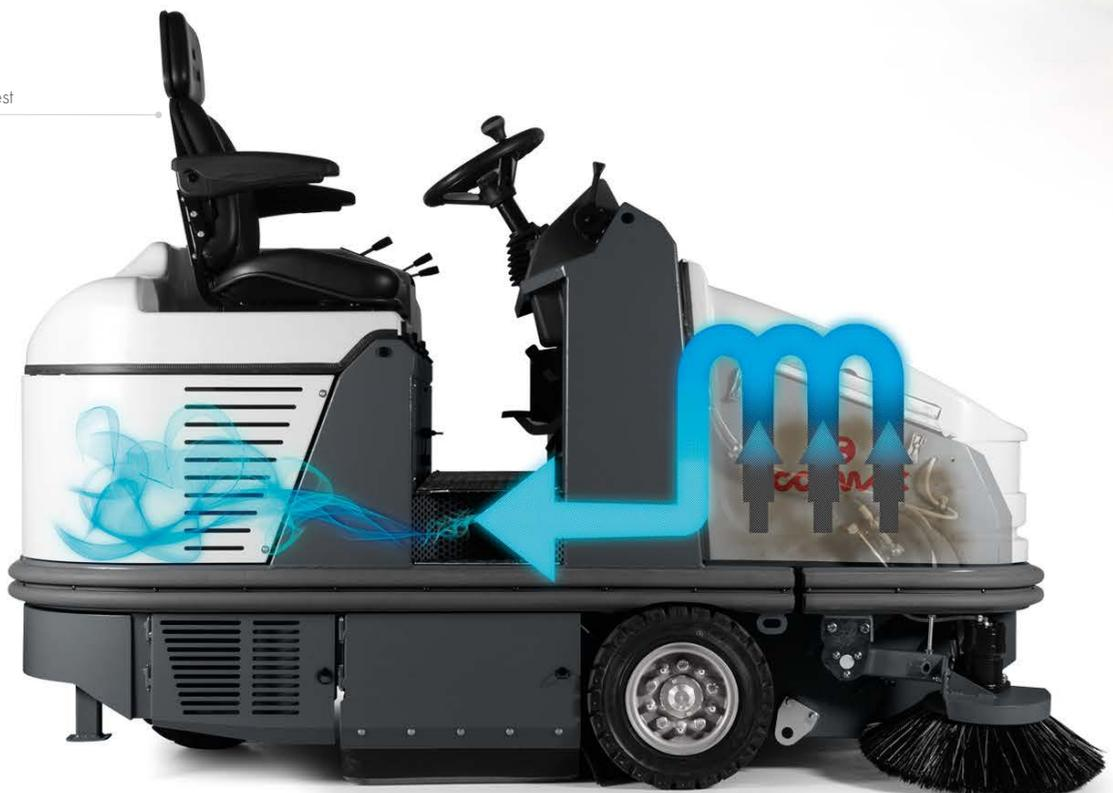
The vacuumed air is discharged through grilles located high up on the machine. This means that none of the dust that has settled on the surface surrounding the machine is lifted, thus guaranteeing excellent cleaning results.
